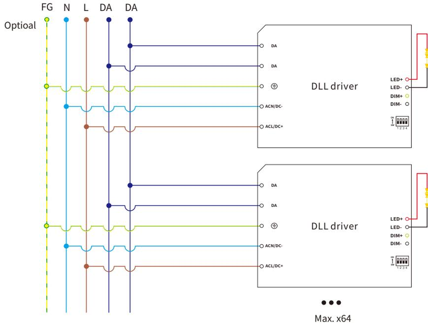
**Switch to the DALI dimming mode**
