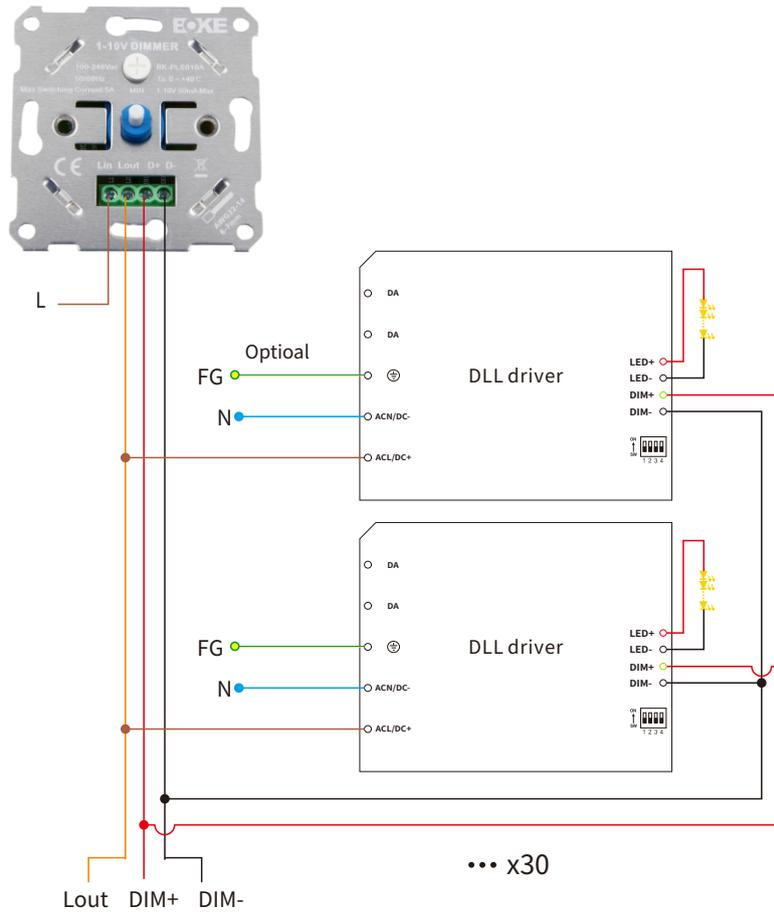
**Switch to the 1-10V / 10V PWM dimming mode**
