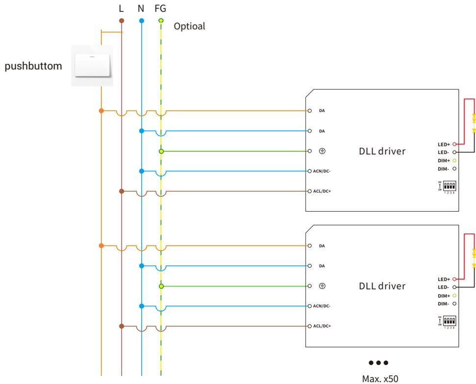
**Switch to the pushDIM dimming mode**
