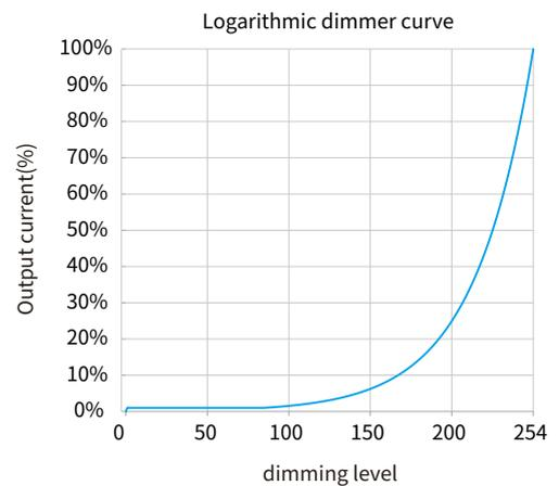
Remarks: The dimming curve can be selected by DALI configuration. The default is logarithmic dimming curve.
