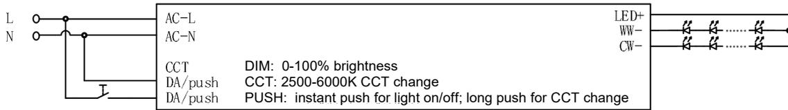
**⚠ Remark:** when using the PUSH dimmer for brightness change or CCT change, please connect AC-L and AC-N FIRST, and then connect the PUSH dimmer to AC-L and CCT terminal.
