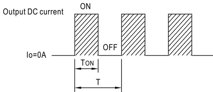
$$\text{Duty cycle(\%)} = \frac{T_{ON}}{T} \times 100\%$$
